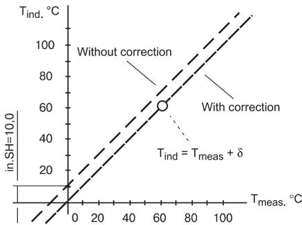
Figure 3. “Characteristic shift” adjustment
