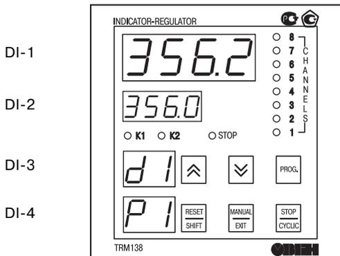
**Figure 15. Instrument front panel**
