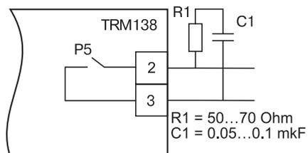
**Figure 10. Relays' contacts connected in parallel at operation under inductive loads**
