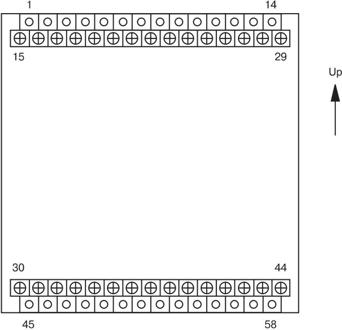
Figure A2.1. Instrument terminal block contacts arrangement diagram
