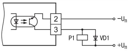
**Figure 11. Application of transistor optocoupler for control over electromagnetic relay assembly**
