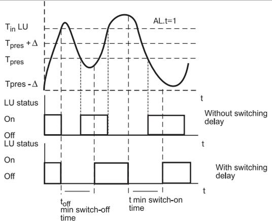
**Figure 8. LU operation with the preset holding time**
