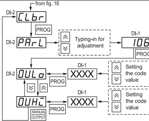
Figure A5.8. Diagram for DAC adjustment
