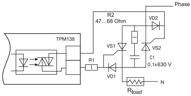
**Figure 13. Triac optocouplers applications for load control by means of a power thyristors**
