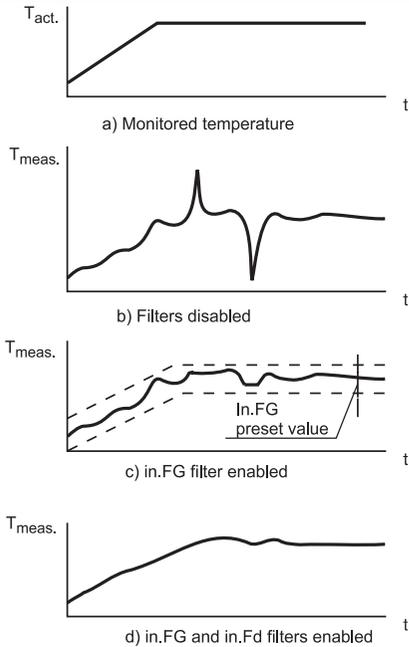
**Figure 2. Digital filters operation timing waveforms**
