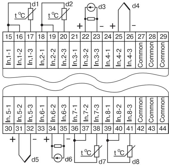
Figure A2.10. Example of connection of various type transducers
