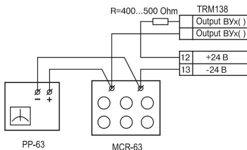
**Figure A5.7. Connection diagram for the equipment during adjustment of the DAC.**
