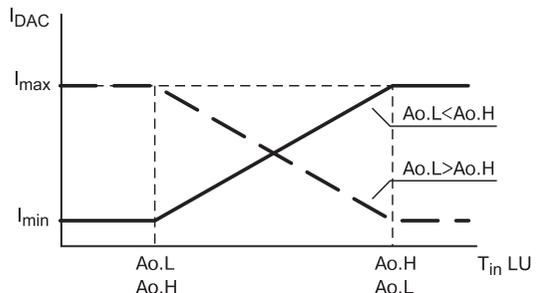
**Figure 9. DAC output characteristics**
