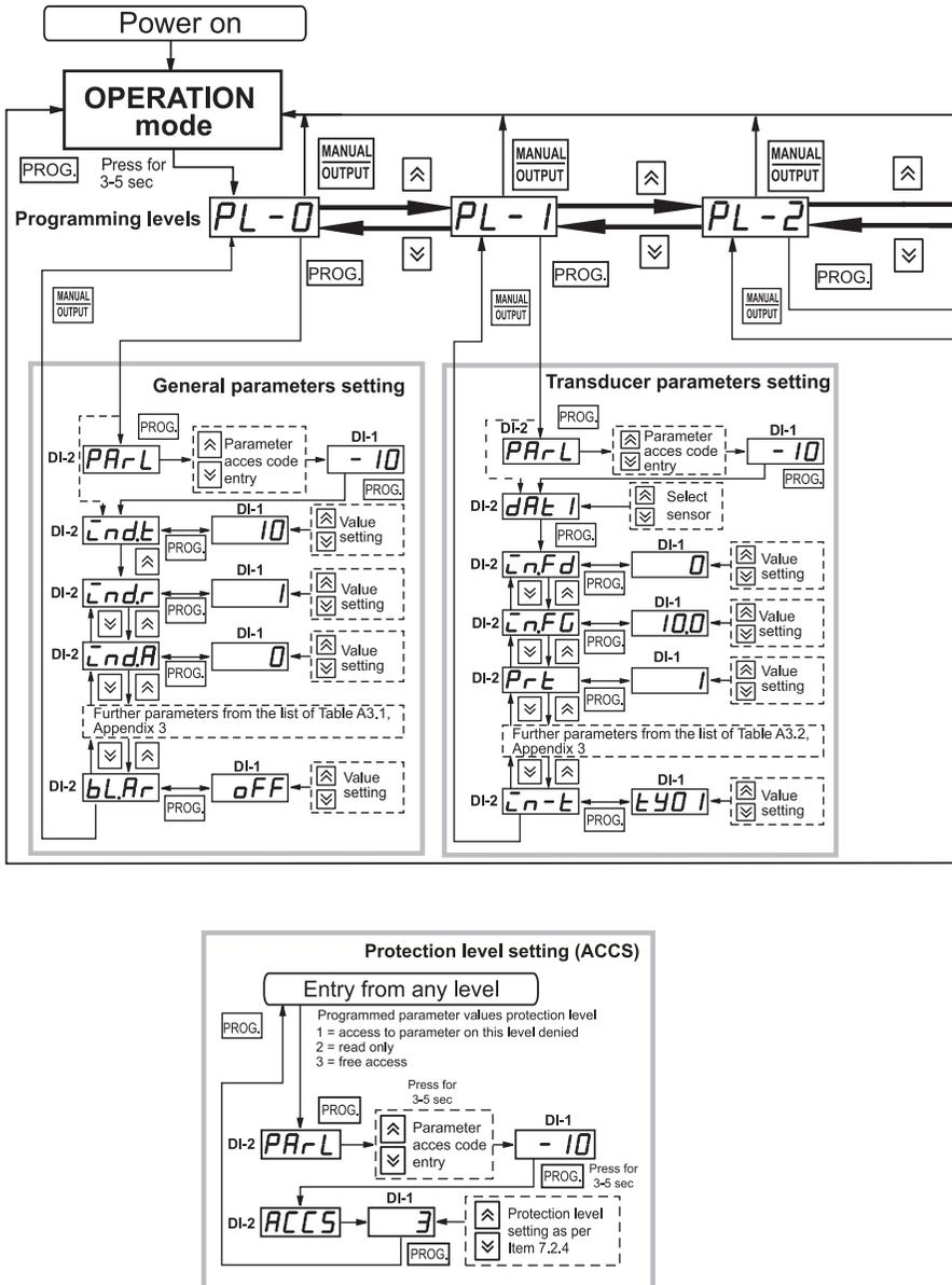
Figure 16. Programmed parameters setting diagram
