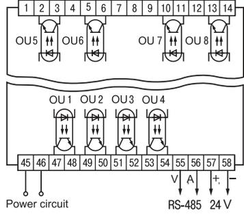
Figure A2.3 Connection diagram for optocouplers in TRM 138-R type instrument
