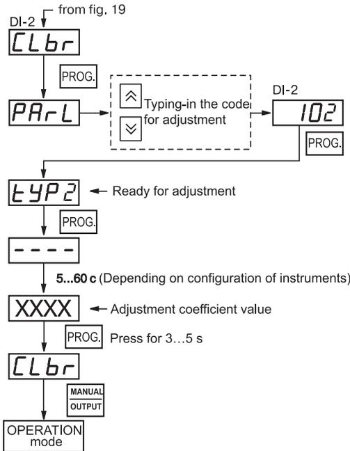
**Figure 5.6.4. Diagram for adjusting thermal couple free ends transducer**
