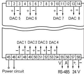
Figure A2.5 Connection diagram for DAC in TRM 138-I type instrument
