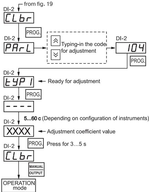
**Figure A5.2. Diagram for adjusting the instrument for operation with a sensing device**
