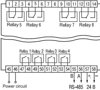
Figure A2.2 Connection diagram for electromagnetic relay in TRM 138-R type instrument
