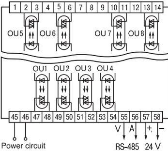
Figure A2.3 Connection diagram for symistor optocouplers in TRM 138-C type instrument
