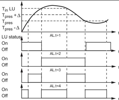
Figure 5. Comparators' output characteristics
