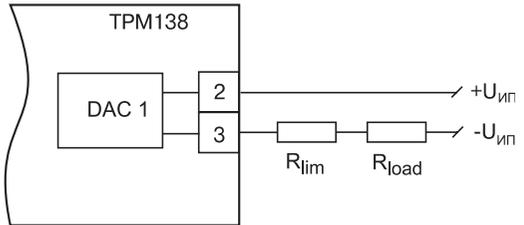
**Figure 14. The DAC / load connection diagram**
