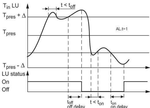
Figure 7. LU operation with reaction and falling delays
