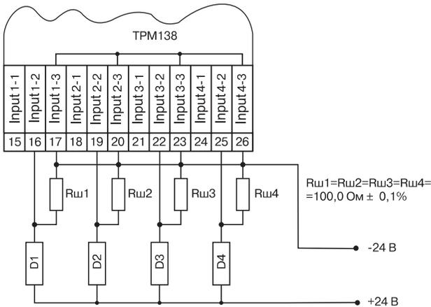
**Figure A2.8 Connection diagram for active transducers d1...d4 with 4...20 mA output signal**
