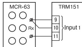
**Figure A5.1. Connection diagram for resistance box during adjustment**
