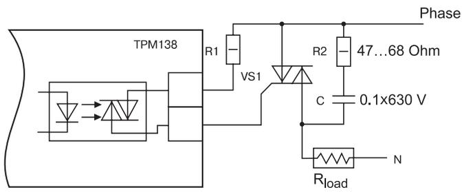
**Figure 12. Triac optocouplers applications for load control by means of a power triac**
