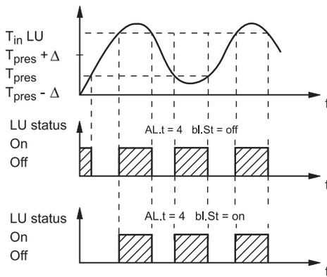
Figure 6. LU operation diagrams at various bL.St values
