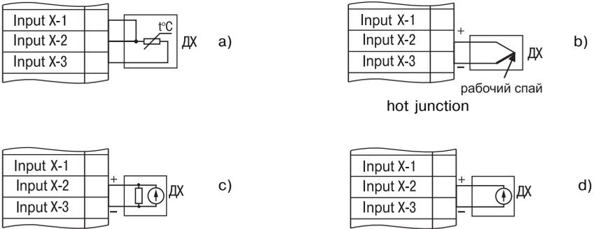
**Figure A2.7 Connection diagram for measurement transducers:**
