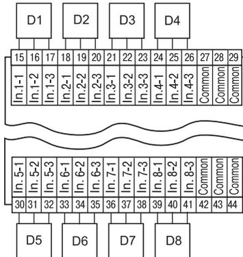
Figure A2.6 Measuring transducers connection diagram
