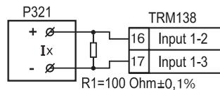
**Figure A5.6. Connection diagram for current calibrator during adjustment**
